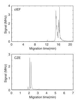
Figure 2. The top trace shows the CIEF separation of ovalbumin (7 nM) and  $\beta$ -lactoglobulin (1 nM). Bottom trace shows CZE separation of ovalbumin (83 nM) and  $\beta$ -lactoglobulin (34 nM), injected at -5 kV for 2 s.
