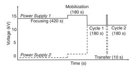
**Figure 1**. Voltage program for 2-D CE. Analytes were focused in the first capillary during the 420-s focusing step. After focusing, a series of mobilization and second-dimension separation cycles were performed. In these cycles, sample as transferred for 10 s and then subjected to a 180-s duration second-dimension separation.
